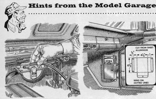
Next time you replace a wiper hose, use clear-vinyl tubing instead of the usual rubber hose. The vinyl won't dry out from heat or soften if oil gets on it. Also, if you see oil in the tubing, you'll know the fuel pump is going bad. Store road maps in a small container screwed to the cowl paneling, and there'll be more room in the glove compartment. Cut the box from do-it-yourself aluminum sheet with household scissors. Bend it along the dotted lines.
