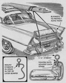
You can tie down loads hauled on the roof of your car safely and conveniently by installing eyebolts on the front and rear bumpers. Drill holes in the bumper or bumper guards and lock each eyebolt in place with two nuts.
