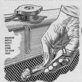
A leak in a radiator can be stopped easily by completely filling the faulty core cell with metal-patching putty or epoxy glue. This won't affect the radiator's efficiency, and it's quicker than trying to locate and solder a pinhole.
