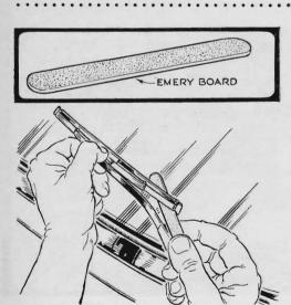
Weather-hardened wipers that smear the windshield can be made to wipe better temporarily. Remove the glaze along the edge with an emery board, nail file, or sandpaper. But remember to replace such wipers as soon as possible.
