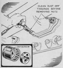
When backing off manifold nuts, rust on exposed threads often jams a nut half-way off the stud. To avoid this, clean the threads with a die *before* removing the nuts. A socket fitted with a setscrew makes a long-reaching die holder.
