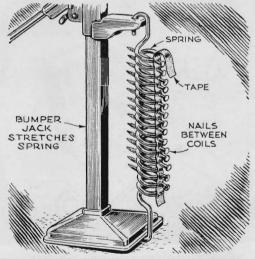
**Installing hood springs** can be made easier if you first stretch them and slip nails through masking tape to keep the coils spread. After attaching the springs, lower the hood slightly to stretch them and pull the tape to release the nails.
