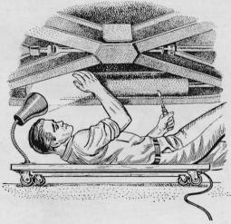
This under-car creeper has a built-in light to illuminate the work area as you move around beneath the car. The gooseneck arm can be adjusted to throw light around corners or behind chassis cross members, leaving both your hands free.
