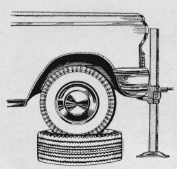
If you must work under a car supported by a bumper jack, take the precaution of placing the spare wheel beneath the wheel that's raised off the ground. If the jack should slip or topple, the spare wheel will keep the car from crushing you.
