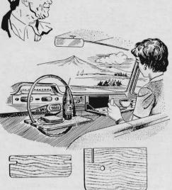
Roadside snacks can be eaten in comfort on these plywood shelves that are stored out of the way beneath the front seat. The shelf shown at left locks firmly on the rim of the steering wheel; the one at right fits over the glove-compartment door.
