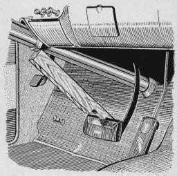
When rear wheels are raised with a jack, the parking brakes become ineffective. To keep the car from rolling, the four service brakes can be applied and held with a stepped stick. Cut several steps and use the one that gives most pedal pressure.
