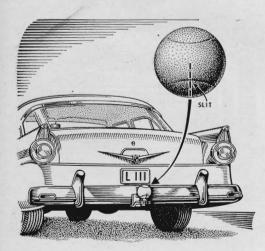
Cap a trailer hitch to keep it out of the weather and free from rust. Slit a rubber ball halfway through and press it over the hitch when not towing the trailer. Don't use grease; it's not needed and will cause the ball to deteriorate.
