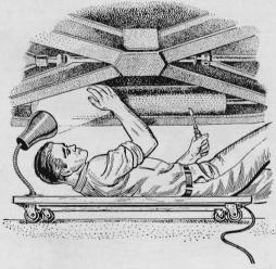
This under-car creeper has a built-in light to illuminate the work area as you move around beneath the car. The gooseneck arm can be adjusted to throw light around corners or behind chassis cross members, leaving both your hands free.
