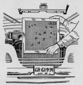
A removable screen to keep insects from clogging the radiator can be made from do-it-yourself aluminum. Make the screen first, then fasten two sections of aluminum channel to the sides of the radiator and slide the screen in the channel.
