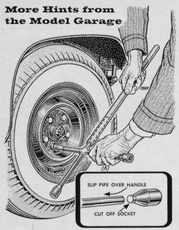
**Loosening wheel lugs** is easy if you have leverage. Cut off the lug-wrench socket next to the one that fits your car. Then slip a two-foot pipe extension over the shaft. Women will appreciate this if they ever have to change a tire.
