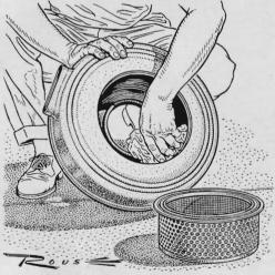
Clean the sump, too, when changing paper air-cleaner elements. Dirt, trapped in the sump after being stopped by the filter, may find its way into the carburetor. Best practice is to remove the whole assembly before taking out the filter.
