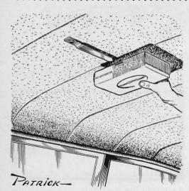
Lift your tissue dispenser—take it out of the glove compartment and put it where both seats have access to it. Fasten one end of a spring to the car ceiling and round the other to slip through slits at the base of the box.
