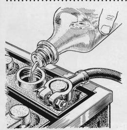
Nursing a parched battery is a cinch if you put the distilled water in an empty pint- or quart-size ink bottle. The nonspill dispensing cap (designed for filling inkwells) lets you pour without waste just the amount your battery needs.
