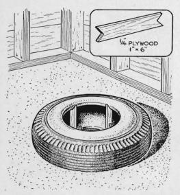
Mounting a new tubeless tire can be difficult when the wrappings have pressed the beads too close together to permit inflation. Let the tire stretch 10 or 15 minutes while the beads are held apart with notched spreaders of the size shown.
