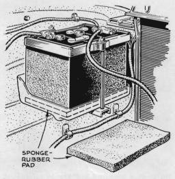
A pad of sponge rubber, ½" thick, will pay dividends if placed in the tray of the battery holder before you install a new battery. It will lengthen the life of the battery by cushioning its ride, and will protect the tray from acid spills.
