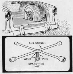
A missing lug wrench is an impossibility if you weld the tool to the retaining nut on your spare-tire stud. Measure outward from the nut to the plane of the tire sidewall; cut a spacer of that length from pipe with an i, d. larger than the stud.
