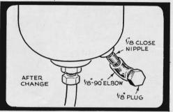
Oil-filter holders often have a small drain plug at the bottom of the case. Usually it's located so far down that it's hard to remove. To make the drain more accessible, attach a close nipple and elbow. Standard 1/8" fittings should work.
