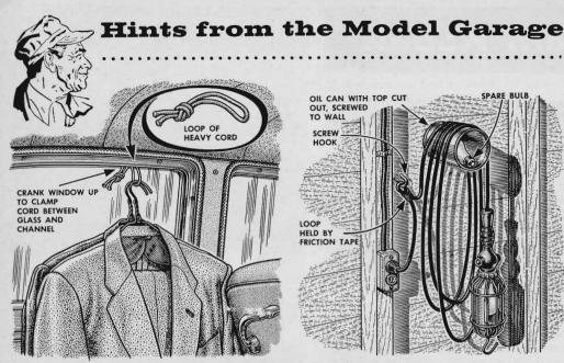
A hanger hook can be improvised in an instant by catching a knotted loop of heavy cord between the top edge of a rear window and its channel. The loop will hold more hangers more securely than the metal hooks used in many cars.
