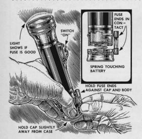
A quick test for car fuses can be made by unscrewing the bottom cap of a metal flashlight and separating it slightly from the body. With the switch on, a good fuse held so that it touches both cap and body will light the flashlight bulb.
