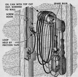
Keep your trouble light trouble-free by coiling it loosely over a tin can nailed to the wall. The can will also hold a spare bulb. Form a loop near the end of the wire and hang it over a hook to keep from accidentally pulling the plug.
