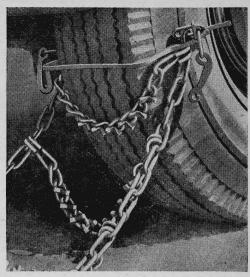
Gadget Helps Put On Chains. A chain attacher made by the St. Pierre Chain Corporation, Worcester, Mass., is illustrated in use above, with the chain stretched out straight behind the wheel and the U-shaped attacher inserted in the side chains and pushed on the tire. The car then is driven forward until the wheel has made one complete revolution and the chain encircles the tire. After the ends are hooked, the job is done. Also in the photo above are special fasteners made by the same company.
