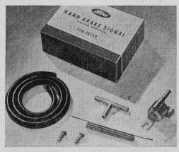
Warns That Brake Is On. A new Ford accessory gives audible warning if you start out without releasing the hand brake. Vacuum operated, it consists of a whistle, a hose and T-shaped unit for connecting to the wiper vacuum line, and a spring to hold the whistle open while the brake is set. It blows only when the engine is running.
