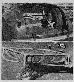
**Trailer Is Collapsible.** A trailer made by Grosch & Gilmore, Milwaukee, Wis., folds up for storage in the car trunk when not in use. Consisting of a canvas body on a tubular aluminum frame, the complete trailer weighs only 45 lb., but will carry a load of 400 lb. It rides on a single pneumatic-tired wheel, mounted on shockabsorbing leaf springs cushioned in rubber. The wheel operates like a caster so the trailer will follow the car. Two ball hitches attach the trailer to the bumper.
