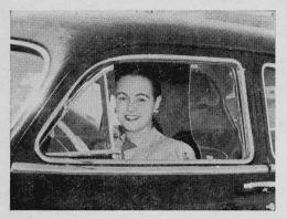
Eliminates Drafts. Even though the front window of a car is wide open, a plastic device made by the NuWorld Products Company, Huntington Beach, Calif., deflects the wind outward, protecting rearseat passengers from drafts. Installed inside the window by three clips, it does not interfere with normal window operation.
