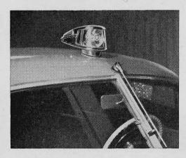
**SPOTLIGHT ON ROOF.** A streamlined movable spotlight for mounting on the roof of a car instead of through the corner post has been introduced by the Trippe Manufacturing Co., of Chicago. Operated by a control knob on the ceiling of the car, the light turns through a field of 270 deg. A switch on the knob turns the light on and off.
