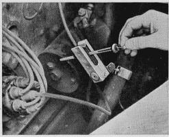
Pads Clean Dip Stiek. A dip-stick cleaner made by Bishman Manufacturing Company, of Osseo, Minn., makes it unnecessary to search for a wiping cloth each time you check the oil. Consisting of two felt pads held together by a spring, the unit may be mounted in a convenient spot.
