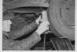
Magnet Forestalls Punctures. Designed to locate nails and other ferrous metals in tire casings, a magnetic tool introduced by Modern Merchandisers, Inc., of Chicago, contains a bulb that glows when the magnet comes near the embedded metal. Said not to be affected by the rim, lugs, or reinforcing wire in tires when properly used, the device is furnished as either a self-contained battery model or for 115 volts.
