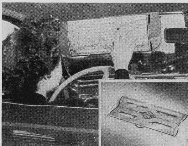
**MAP HOLDER FITS ON VISOR.** Attached to the car visor with a strong elastic cord, the holder shown above makes it possible to keep road maps, guide books, and other reference material within easy reach and sight while driving. Produced by Visor-Ads, of West Hartford, Conn., the device is made with a clear plastic front, reinforced with steel wire to increase its durability.
