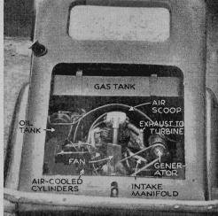
claims that power is increased through a "turbine" method of bringing the heat and pressure of the exhaust gas into play. Built with no frills, not even an extra wheel, the car weighs approximately 1,200 lb. A roomy luggage compartment is located under the hood and a single headlight is centered in a dummy radiator.
