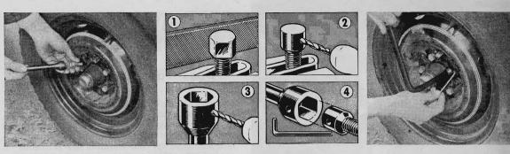
**TIRE THEFT** is made extremely difficult if you make use of the simple procedure outlined in the photos and drawings above. In principle, the method consists of rounding one tire-retaining nut or bolt so that it cannot be turned by a lug wrench without a special key. The idea is adaptable either to the nuts or the bolts variously used with pressed-steel wheels.
