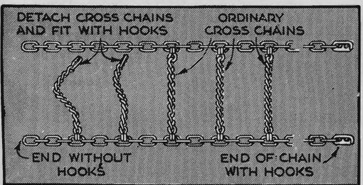
**3 EVER GET STUCK** because you couldn't jack up the car to put on chains? One way to apply full chains without moving or jacking the car is to fit two or three of the cross chains at one end with hooks instead of links, as shown in the drawing. These hooks can be detached when you're in mud or snow and the ends of the chain can be joined. Rehook them on firm ground.—B. W. P.
