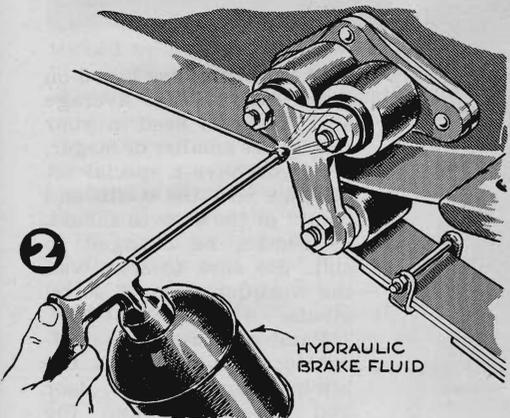
**2 SQUEAKING RUBBER BUSHINGS** and shackles on the ends of springs, shock absorbers, and the like are a particular nuisance to many drivers who know they can be oiled only at the risk of rapid deterioration of the rubber. Hydraulic-brake fluid sprayed on them, however, is not harmful to the rubber, and it lubricates sufficiently to cure the most persistent squeak.—J. C.
