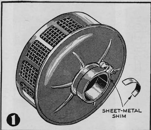
**1 CARBURETOR AIR FILTERS** rattle like flivver fenders when they become loose and, worse luck, they let in unfiltered air. In time, too, the clamps holding them have a tendency to distort so that tightening is useless. A repair to make them tighten evenly and to stop further distortion can be made with a steel shim put on under the clamp as shown in the drawing.—R. R. K.
