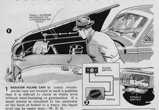
2 A SECRET RADIO SWITCH will prove handy in circumstances where a car must be left unlocked, as in many parking lots or garages. A toggle switch, wired in series with the regular radio switch and installed in the glove compartment (which in most cars can be locked), will help prevent this annoying battery drain.—R. W.
