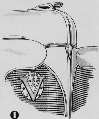
**1 BREAKS IN GRILLS** can be concealed by mounting radiator emblems over them. To do this, drill suitably spaced holes in a piece of flat stock such as heavy sheet metal and place this behind the bars of the grill, running the mounting screws through it.—J. B.
