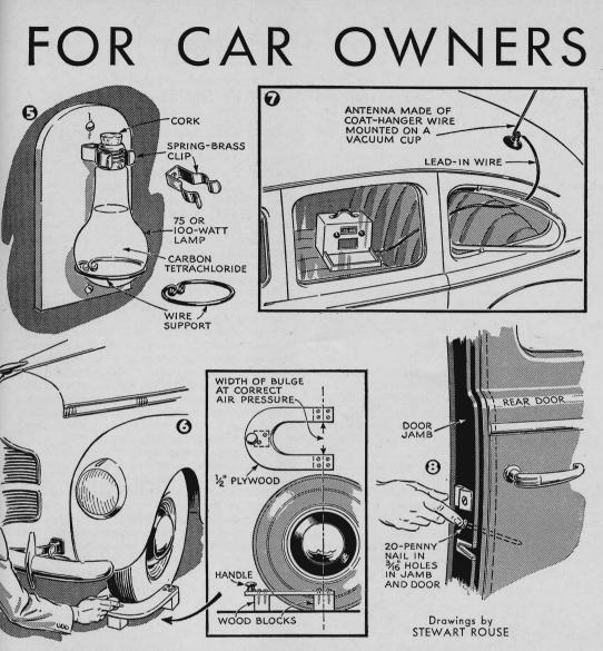
**5** A FIRE EXTINGUISHER for your car can be made simply out of an old 75 or 100-watt electric light bulb. Saw off the inside of the base and remove the porcelain. Then break the end of the glass bulb in the base and shake out the inside parts. Fill with carbon tetrachloride, leaving space for expansion, seal with a cork, and mount under the dashboard. To use, throw the bulb hard at the center of the flames.—W.A.E.
