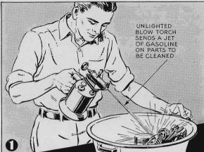
CLEANING DIRTY GEARS and engine parts to which grease, sludge, and gummy deposits are clinging is simplified with a blow torch which has been filled with gasoline and pumped up to full pressure. Place the parts to be cleaned in a pan or a clean pail, and open the torch jet so that it shoots a stream over the dirty surfaces.—C.L.R.
