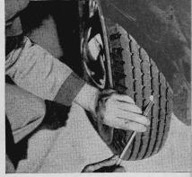
Sharp stones, nails, tacks, and other objects should be removed promptly before they cause damage. Never drive a tire against or over the curb
