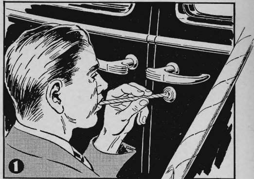
STUFF END OF SODA STRAW WITH FLAKE GRAPHITE, THEN FLATTEN
