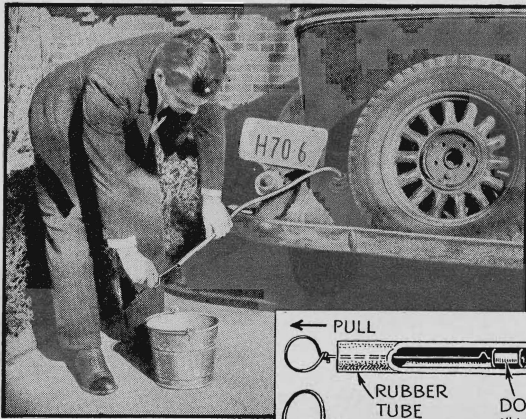
A jerk on the plunger starts siphoning action. Drawing at right shows its simple construction
