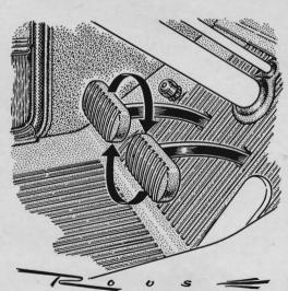
**Rubber pads** on clutch and brake pedals that show wear on one side can be turned upside down or switched on the pedals to distribute wear. The pads will last longer and there will be less danger of your foot slipping off a worn corner.
