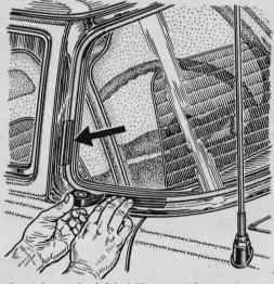
**Leaking windshield?** A quick repair can be made by sealing the gap between the glass and the rubber gasket with plastic electrician's tape. Applied carefully and left undisturbed, the tape makes a permanent repair that doesn't look patched.
