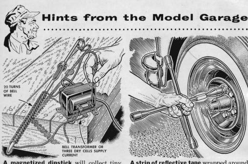
A magnetized dipstick will collect tiny iron and steel particles in a crankcase. Magnetize it with a quick pulse of current through a temporary coil. With AC you may need to repeat until you catch the current cycle at or near a peak.
