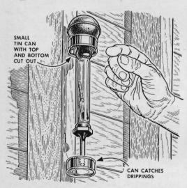
**Store a hydrometer** safely in a dripcatching hanger made from two small tin cans nailed to a stud. The upper can has its bottom cut out, forming a holding ring. The lower can is used with its bottom intact to catch drippings.
