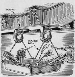
Keep tools and small parts handy in a tray supported by two husky magnets. They'll stick almost anywhere under the car and can be quickly removed and shifted elsewhere. Fasten the magnets to the tray at each end with brazing rod.
