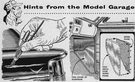
Feed drops of paint neatly to a touch-up brush by taping an eyedropper to its ferrule. Place the tip of the dropper a little below the ferrule so that paint will flow onto the top of the bristles and work its way evenly to the tip. Cover worn interior panels—especially those under the dash—with pieces of embossed sheet aluminum. Simply pry off the old panel and cut the aluminum to fit it, allowing enough extra on all sides to bend over the old panel.
