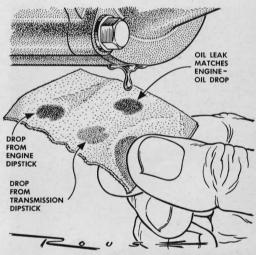
To locate an oil leak, pull the dipsticks from engine and automatic transmission and let a drop of oil from each fall on a white blotter. Then hold the blotter under the car to catch a drop of leaking oil. Compare the colors.
