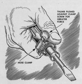
**Get a better grip** on the handle of a screwdriver by tightening a worm-gear hose clamp around the handle near the shank of the blade. Grasp the tool so that your thumb bears against the clamp screw in the direction you're turning.
