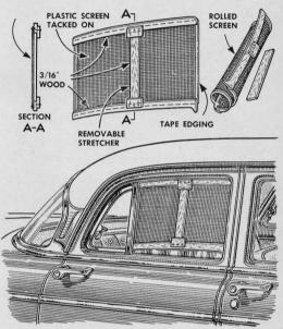
These car screens roll up for compact storage when not in use, yet they can be installed in minutes. Tack plastic screen to an upper and lower spreader shaped to fit the contour of the window. Insert a strip of wood to stretch the screen and secure it by raising the window against it.
