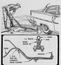
Flush dirt from the underside of a car without getting yourself wet by clamping the hose to a dolly made from a 6' length of pipe and half a roller skate. Bolt the skate to the pipe and bend up a handle. To avoid a geyser, turn on the water after pushing the dolly under the car.
