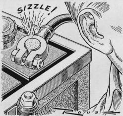
A frying noise from this battery terminal was the only response when the starter switch was depressed. The cable seemed tight. But the mechanic found it was making only slight contact with the post. Cleaning completed the circuit.
