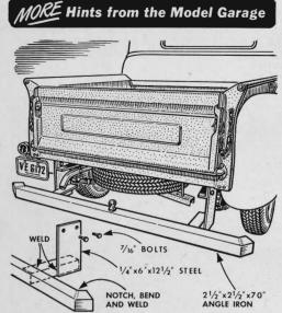
This welded angle-iron bumper doubles as a trailer hitch and rear step for a light pickup truck. The assembly was welded to 4" steel plates bolted to the truck's frame. The ends were shaped by cutting a V notch, bending the angle, and then welding the joint. A ball hitch for a trailer was mounted in the center of the bumper.
