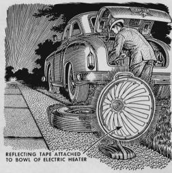
A roadside reflector can be made from a discarded electric heater of the reflector type by covering the concave surface with luminous paint or strips of reflector tape. It makes a neater job if you first remove the wiring and old heater element.
