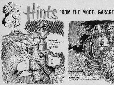
In making a gasket, you can locate and cut bolt holes in one step with a steel ball slightly larger than the hole. Cut the gasket to shape and place it on one surface to be joined. Tapping the ball lightly over the hole makes a clean cut.
