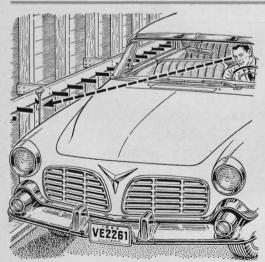
Installing a guide rail on the opposite garage wall helps you leave room to get out on the driver's side. When the fender guide on your car just touches flexible fingers cut to length from an inner tube, there's room to open the other door, too. Insert fingers in saw slots in a one-by-three.
