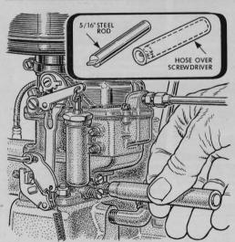
This screwdriver stays aligned with carburetor adjusting screws while you give your full attention to tune-up jobs. Make the screwdriver from 5/16" rod and draw on a tight sleeve of rubber hose with a 4" extension to fit over the screwhead.
