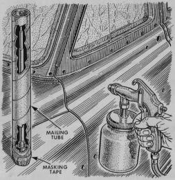
A mailing tube can save you the trouble of masking your car's radio antenna next time you want to do a partial or complete body refinishing job. Just slip the tube over the end of the telescoped antenna.
