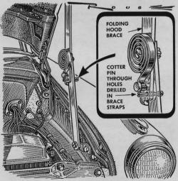
A hood that is supported by tension springs may develop a habit of falling when the springs weaken. To make it safe, drill a small hole through the brace straps with the hood up. A cotter pin slipped in the hole will then keep the hood from falling.
