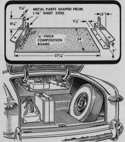
**Small packages** will be kept out of harm's way in a luggage compartment if you build a light shelf like this one. It is attached to the hinge guards by bolts and wing nuts so that it can be removed when you need maximum space. The dimensions given suit a 1951 Ford but can be adapted to other cars. Be sure to leave clearance for trunk lid.
