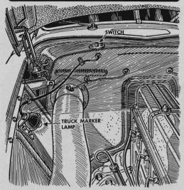
An under-hood light is easy to install. Buy a truck marker lamp from an autosupply store, remove the red glass and bolt the light to the side of the engine compartment. Aim it to shine on the dipstick. Then mount a car-door switch so that the descending hood will turn it off. Run a lead to a hot wire and the job is done.
