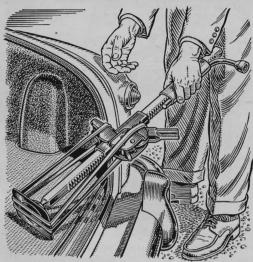
Inner Tube Quiets Jack. A bumper jack won't rattle so much in the trunk if you store it this way. Raise the jack a few notches against an inner-tube rubber band. Cut a sleeve from a bicycle inner tube, pull it on the shaft, and slip in handle.
