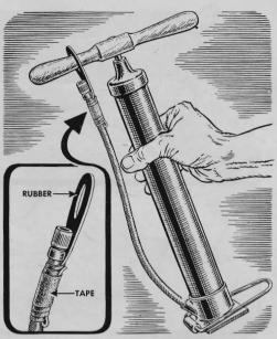
A piece of rubber attached to your tire pump like this will keep it a compact unit while stored with other gear in your car. The projecting rubber bends aside and doesn't interfere when you screw the air hose to the tire valve.
