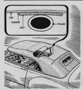
A convertible top often wears through at the points where the fabric slaps the frame cross members. A strip of felt or cloth attached under the top above these members will give the fabric longer life. Use rubber cement to attach the strips.
