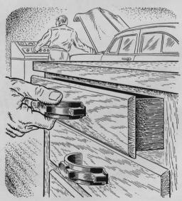
**Discarded caps** from the big ends of connecting rods can be put to use as drawer or cabinet-door pulls in a shop. Bolt or screw them in place. A garage that makes general repairs will usually have a lot of the caps around.
