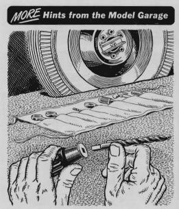
A twist drill is a worthwhile addition to a car tool kit if you consider a regular hand drill too bulky to carry. One idea is to grind the drill shank so that it can be used in the handle of a screwdriver that has a set of removable blades.
