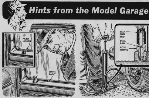
Paint Shows Button Position. From a distance it is sometimes difficult to tell whether car-door lock buttons are up or down. To remedy this, pull them up and paint a white strip around the base. If strip doesn't show, the door is locked.
