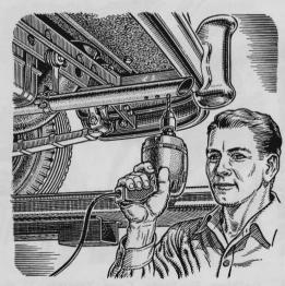
Drilled Holes Drain Tailpipe. You can retard corrosion of a tailpipe by drilling three 3/16" holes 1" apart at the exhaust end, as shown here. The holes will give condensed water a better chance to drain out of the pipe.
