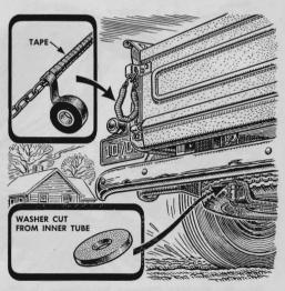
Curbing Truck Noises. Tail-gate chains on a trailer or light truck can be silenced by winding them with tape. If a spare-tire lock like the one shown rattles because of play between the lock and receptacle, insert a rubber washer to take up slack.
