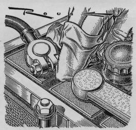
Wipe off dirt and moisture from the top of your battery occasionally. If too much piles up, it will form a leakage path between the terminals. Another tip: clean out the small vent holes in the plugs with fine wire from time to time.
