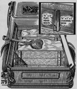
Sand and gravel or other different materials can be carried in a small truck at the same time without mixing if you divide the body like this. Install matching pieces of channel iron on opposite sides of the body. Cut division boards to slip into the channels. It may help to space each division to hold one cubic yard of material.
