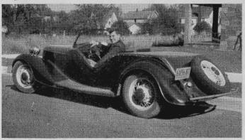
This slick job is the work of Carl Pierce, Cortland, N. Y. Basically a 1934 Ford coupe lowered to 8" road clearance, it has a souped-up 1939 Ford engine. For more responsive steering, the pitman arm was lengthened so the wheel makes only two turns from lock to lock. Brakes are 1940 Ford hydraulic, instruments are from a 1936 Cadillac.
