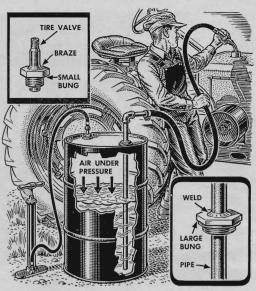
Air Pumps Fuel from Drum. It takes only simple equipment to pump gasoline from a 55-gallon drum. Give the tire pump a few strokes and the pressure will raise the fuel quite a distance. It's best to have a shut-off nozzle on the gas hose.
