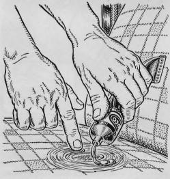
**Cement Saves Seat Covers.** If seat covers are about to wear through, apply a thin coat of Duco cement on and around the worn area. D. Earl Chase, of Long Beach, Calif., says he has extended the life of covers a year or more by this trick.
