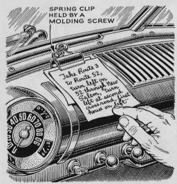
Clip Will Hold Notes. An ordinary spring clip mounted like this makes it easy to keep notes in sight while driving. Remove one of the screws from the windshield molding, slip it through the eye of the clip, and replace in the molding.
