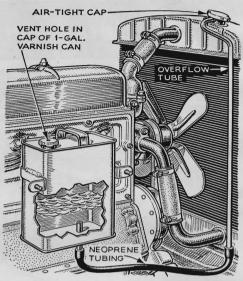
**Save Your Antifreeze.** In cars with atmospheric cooling systems, you can lose alcohol antifreeze through the overflow pipe when the engine runs hot. A tank like this will save it. Boiled-out alcohol will condense in the can. When the engine cools, vapor in the radiator will condense, sucking alcohol back from the can.
