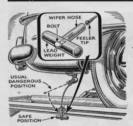
Watch Out for Curb Feelers. When a car is on a hoist for a lube job, the new curb feelers are at just the right level to jab an unwary worker in the eye or face. To eliminate this hazard, Marion L. Rhodes, of Knightstown, Ind., keeps on hand a couple of weights made as shown in the sketch above.
