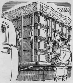
Rubber Holds Truck Cover. To save time in lashing a tarpaulin over a stake body, cut rubber bands from an inner tube and tie one to the end of each rope. Then you can slip the rubber band on or off the hook instead of tediously tying or untying the rope. The elastic keeps the ropes and cover tight.
