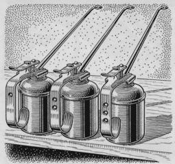
Holes Identify Grade of Oil. In some shops it's common practice to keep several similar pump oilers filled with oil of different grades for different jobs. To avoid mixups, Marion L. Rhodes, of Knightstown, Ind., suggests drilling identifying holes in the handles—one for No. 10, two for No. 20, and three for No. 30.
