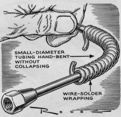
How to Bend Tubing. In replacing an oil or gas line, you usually have to make several short-radius bends in the tubing. To keep the tubing from collapsing, Frank M. Butrick, of Alma, Mich., suggests first wrapping it at the bend point with a piece of wire solder. Remove the solder after making the bend.
