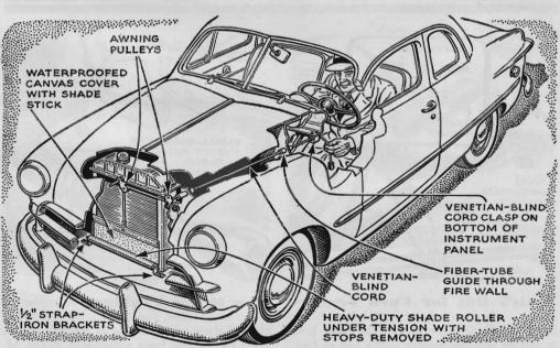
Radiator Cover Warms Engine. When the thermometer dips toward zero, an adjustable radiator cover will give your engine a nice boost. Donald Richards, of Brooklyn, N. Y., installed this one after finding he got little benefit from his hot-water heater on cold days. The cover can be adjusted while driving.
