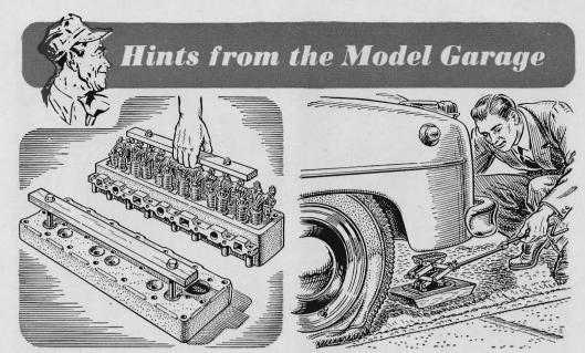
Lifting an Engine Head. A cylinder head is always a clumsy object to handle. A wood lifting bar makes the job easier. For an overhead-valve engine, drill holes in the bar to suit the studs that hold the rocker-arm cover. For a big L head, run bolts through properly spaced holes and thread into the end spark-plug holes.
